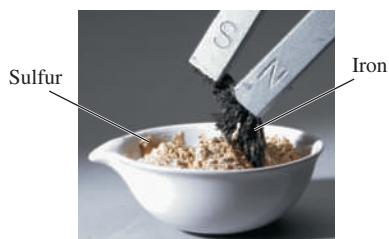
FIGURE 1.5 Iron pyrite is composed of the elements iron and sulfur. Iron is magnetic and can be separated from sulfur when the two exist as elements mixed together. Iron pyrite, a compound of iron and sulfur, is not magnetic.
